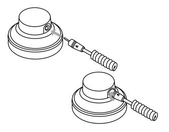
In order to lock your selected cable into the Pro Set 3 you simply insert and twist to lock.
